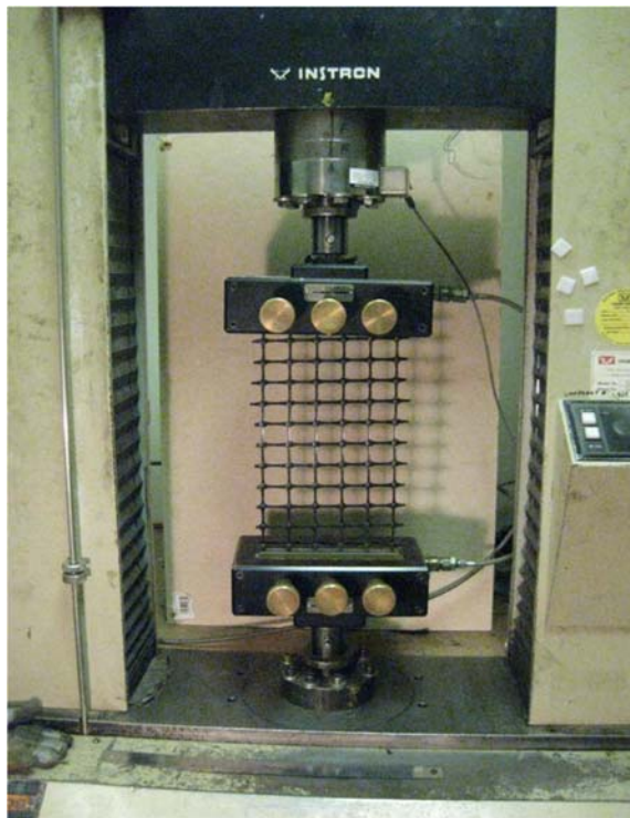
(a) Tensile Test Setup for Geogrid
