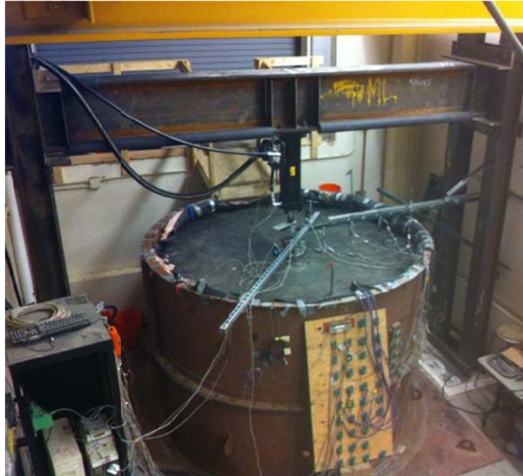
Figure 4.16. Completed Large-Scale Test Setup for Flexible Pavement Experiment
