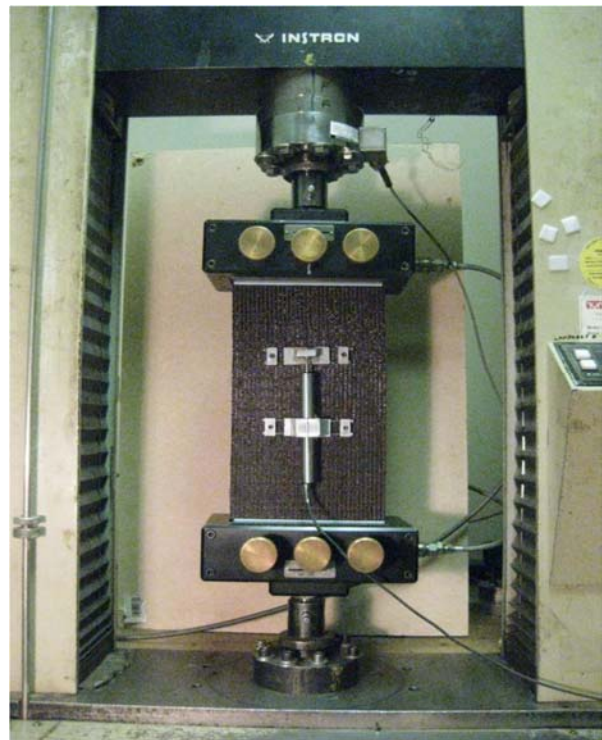
(b) Tensile Test Setup for Geotextile
