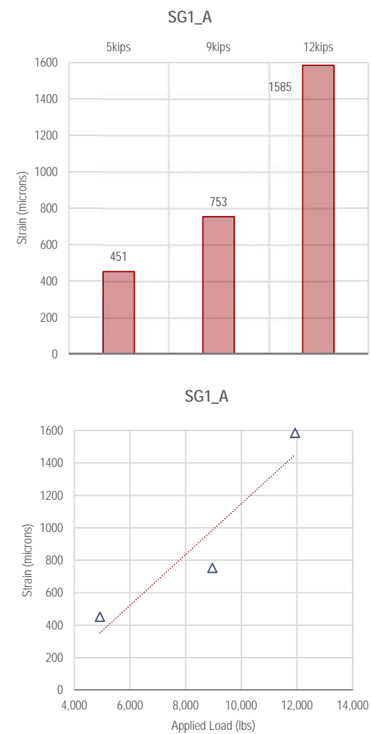
Figure F4-22. Summary of SG1_A measurements—Static Loading
