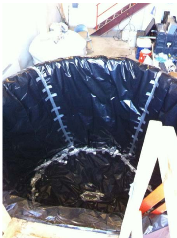
Figure 4.15. Plastic Sheet Covering the Wave-Absorbing Material in the LST
