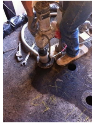
Figure L-9. Coring of the asphalt concrete layer in the LST
