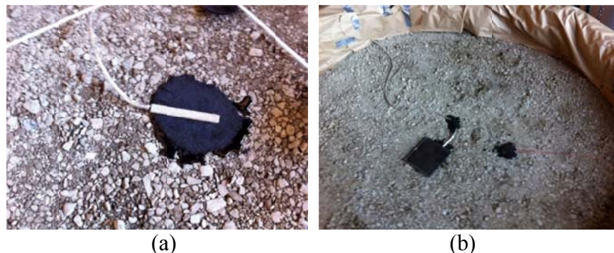
Figure 4.20. (a) In-Place Asphalt Strain Gauge; (b) Final In-Place Asphalt Strain Gauge with Temperature Sensor
