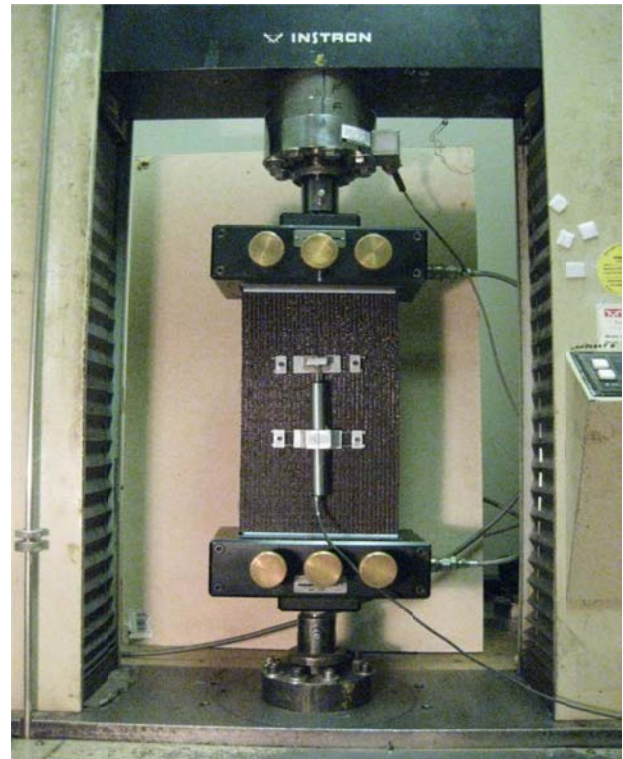
(b) Tensile Test Setup for Geotextile
