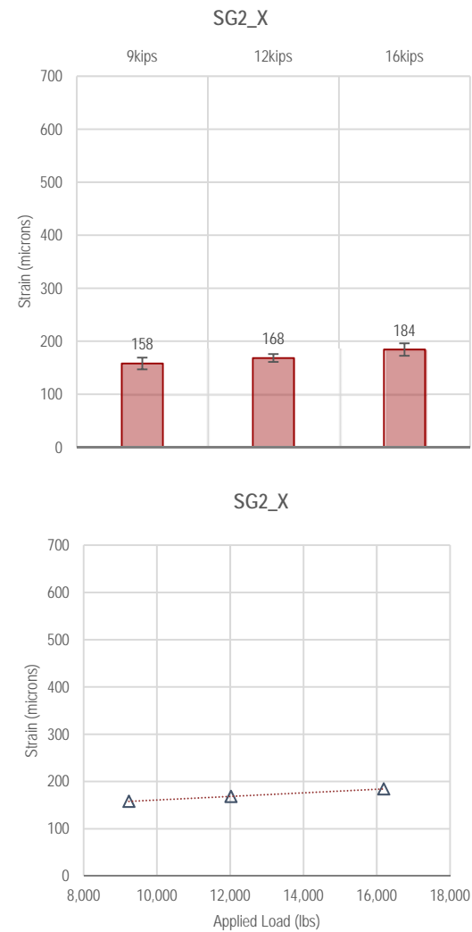
Figure F1-16. Summary of SG2_X measurements—Dynamic Loading
