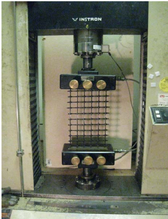
(a) Tensile Test Setup for Geogrid
