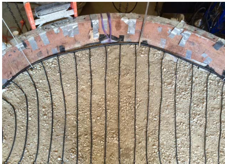
Figure L-11. Completed irrigation system: soaker hose configuration
