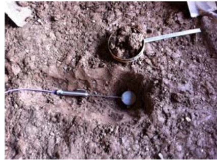
Figure 4.19. Placement of the 4-inch Earth Pressure Cell in the Subgrade
