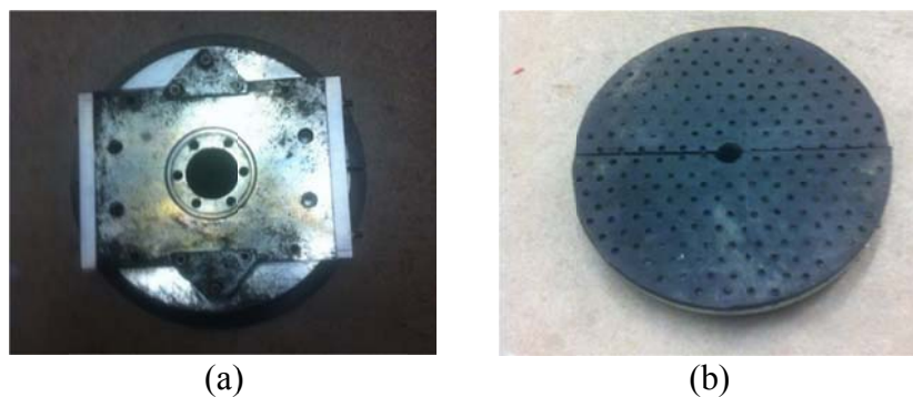
Figure 4.14. FWD Loading Plate Used in the LST Experiments: (a) Top View; (b) Bottom View
